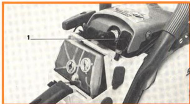
The intake air preheating kit prevents the air filter and carburetor becoming iced in very cold weather and also stops snow entering the fan housing.
