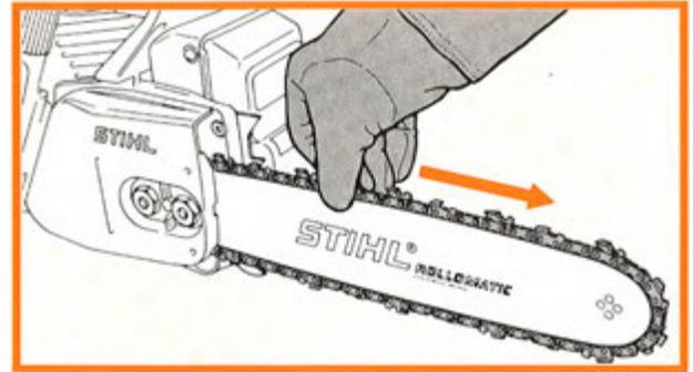
The Oilomatic chain is correctly tensioned when it fits snugly against the underside of the bar but can still be pulled easily along the bar by hand (with chain brake disengaged). Important: Wear protective gloves when performing this work.
