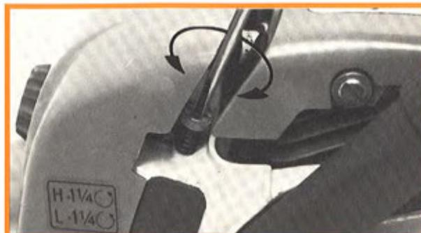
engine speed will be exceeded. This can cause engine damage, brought about by lack of lubrication and overheating in particular. Corrections to the setting of the high speed adjusting screw may be carried out only if an accurate tachometer is available to check the maximum engine speed of 13,000 r.p.m. (12,500 = 028 WB) (with bar and correctly tensioned chain).
