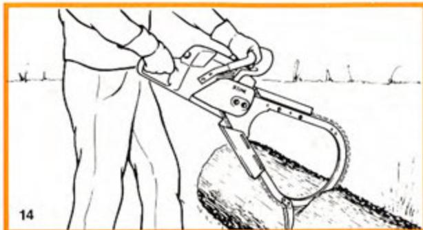
The spurs should always be placed firmly against the wood before starting a cut (ill. 14) and should be kept against the wood until the cut is completed. Failure to keep the spurs firmly against the wood during the entire cut could cause the saw to react violently and could result in serious injury or death to the operator.
