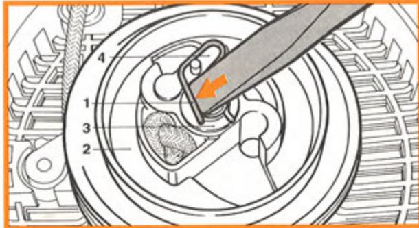
Now insert the pawl (4) in the rope rotor (2) and fit the washer (3) on the starter post. Use a screwdriver or a suitable pair of pliers to press the spring clip (1) onto the starter post, making sure that the spring clip engages on the pawl's guide pin and points in the clockwise direction. Finish off by tensioning the rewind spring (see below).
